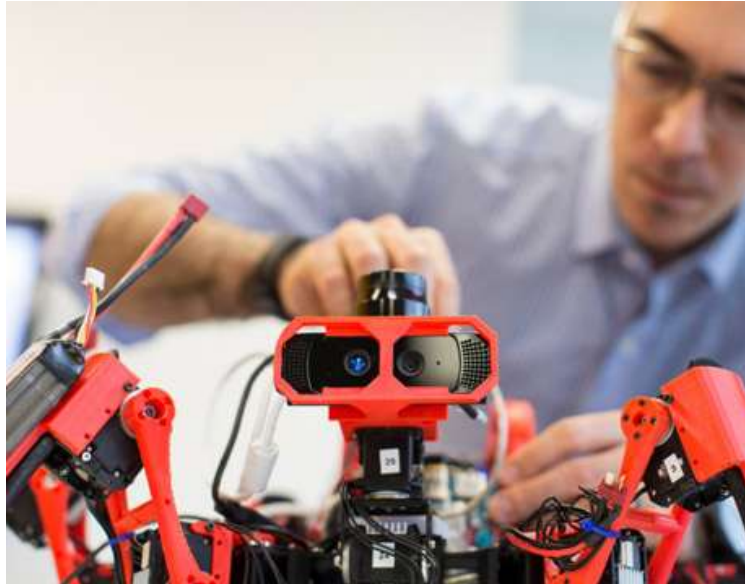
A fully autonomous spider-like robot can 3D print complex structures and surfaces. Image: Siemens
